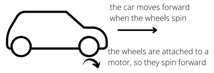
A car is a good example of how we translate the rotational movement (spinning motion) of a motor to linear motion (forward and backwards).
